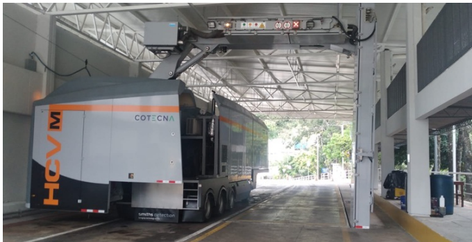
Truck scanner at Anguiatú. Photo shows a large machine capable of scanning an entire truck in a single pass
